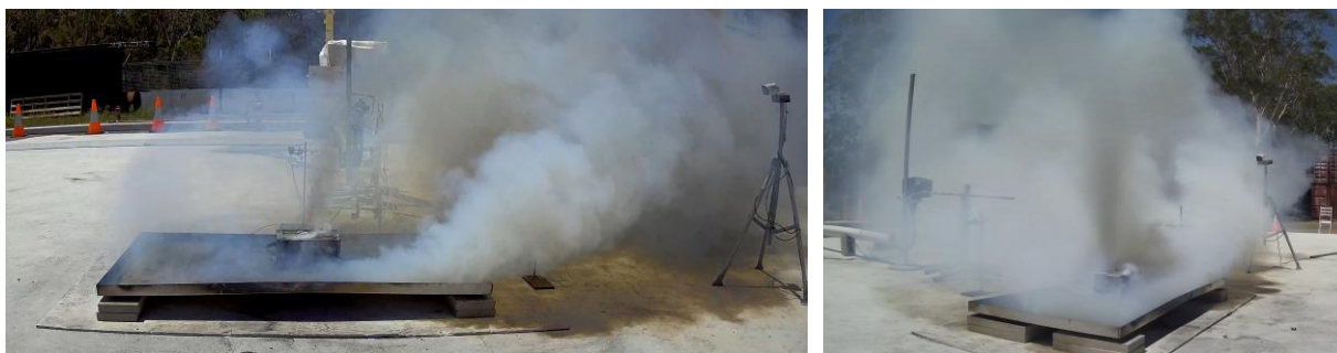
Figure 49. High rate of vapour production from high-pressure venting immediately prior to ignition in test 'Test 32: Steel, Free burn'.
