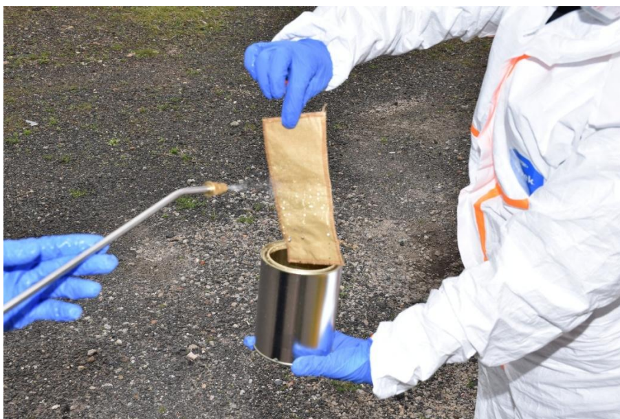
Figure 90. Example image of wet decontamination procedure.
