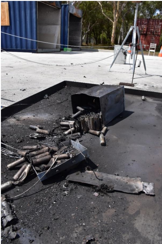
Figure 82. Test 38: Steel, LiB fire blanket showing catastrophic case failure.
