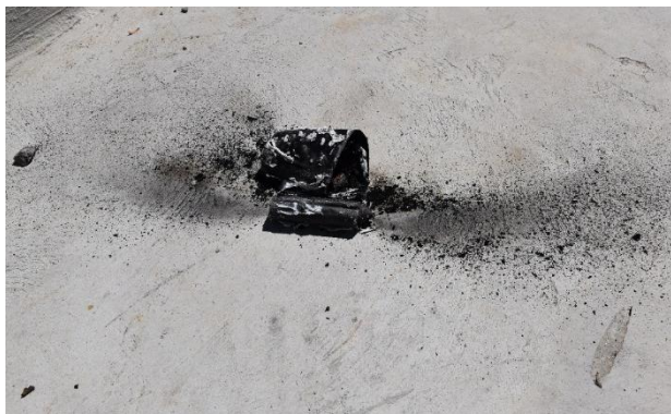
Figure 43. Example of an ejecta classified as a 'Significant Projectile', approximately 13 m from point of origin .
