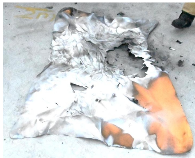
Figure 72. The final position of the blanket and battery at the conclusion of the test and the damage to the blanket ('Test 22: Aluminium, LiB fire blanket').
