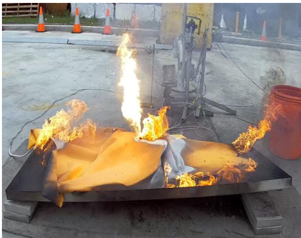
Figure 73. 'Test 23: Aluminium, LiB fire blanket' photo series at distinct timepoints during the test.
