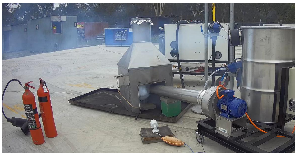
Figure 98. The vapours in the outlet charge at their most visible period in from Trial 1.
