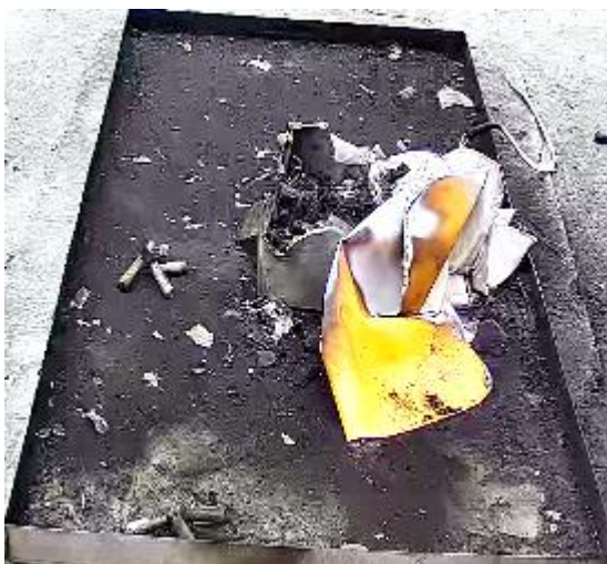
Figure 72. The final position of the blanket and battery at the conclusion of the test and the damage to the blanket ('Test 22: Aluminium, LiB fire blanket').
