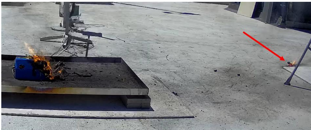
Figure 79. Example of a ‘Significant Projectile’ still flaming 7 s after being ejected from pack.
