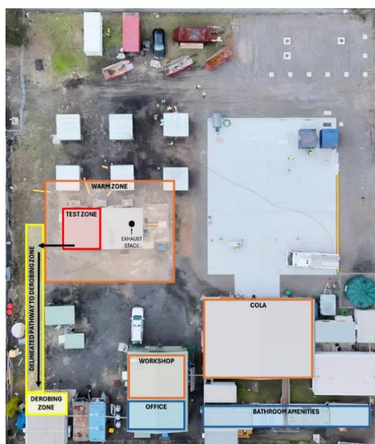
Figure 104. Overhead view of the single cell testing areas and workflow.
