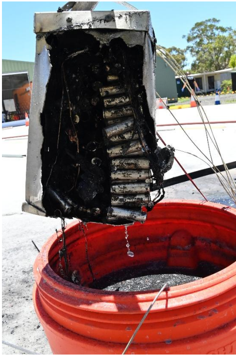
Figure 84. Test 26: Aluminium, Water showing a large hole in aluminium case, representative of majority of tests.
