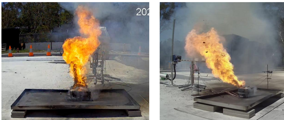
Figure 50. Jet-flaming event from 'Test 32: Steel, Free burn', the shortest duration test.
