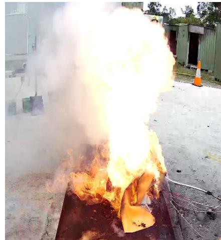
Figure 71. The gas expansion and explosions lifting and moving the blanket ('Test 22: Aluminium, LiB fire blanket').
