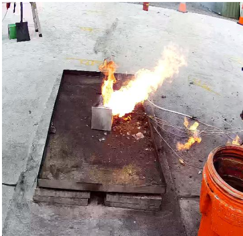
Figure 70. The battery in test 'Test 22: Aluminium, LiB fire blanket' prior to the application of the LiB blanket and 4 s after application, a jet flame burned through.
