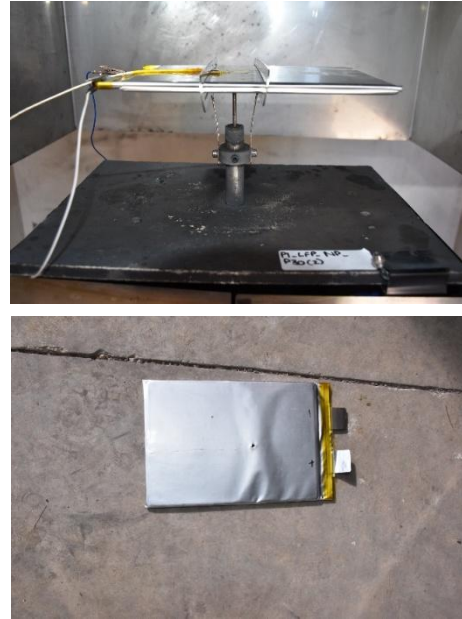
Figure 11. LFP pouch cells at 30% SoC under nail penetration abuse all showed little to no deformation in cell structure. Clear hole where nail has gone into battery can be observed.
