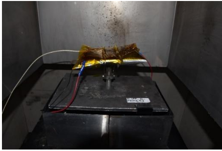
Figure 18. LFP pouch cell at 100% SoC under heating abuse shows the ballooning consistently seen with LFP cells under heating abuse where there was a high build-up of pressure creating a ballooning effect of the cell wall. At the conclusion of the test the cell deflated and went rigid.
