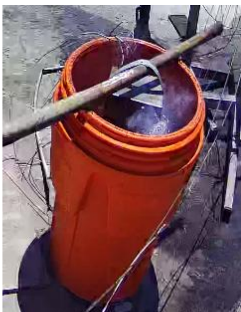
Figure 76. Test ‘Test 41: Steel, Water’ external signs of TR were observed under application of 122 L of water over 2 min 8 s.
