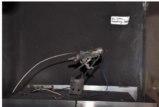
Figure 17. NMC cylindrical cell at 30% under heating abuse. Jelly roll has been exploded out the safety vent end of the cell and test stand sustained damage due to explosive force.
