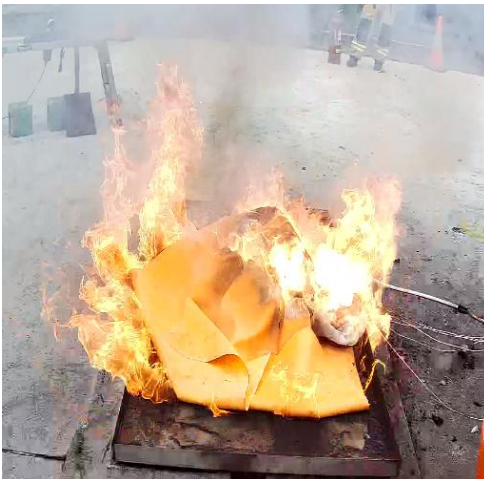
Figure 71. The gas expansion and explosions lifting and moving the blanket ('Test 22: Aluminium, LiB fire blanket').
