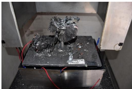
Figure 14. NMC pouch cell at 100% SoC under heating abuse is destroyed - interior has fallen apart
