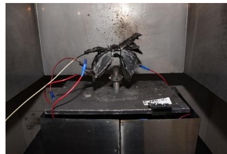
Figure 15. NMC pouch cell at 30% under heating sustained damage with flaming combustion. While heavily damaged, most of the cell remained intact
