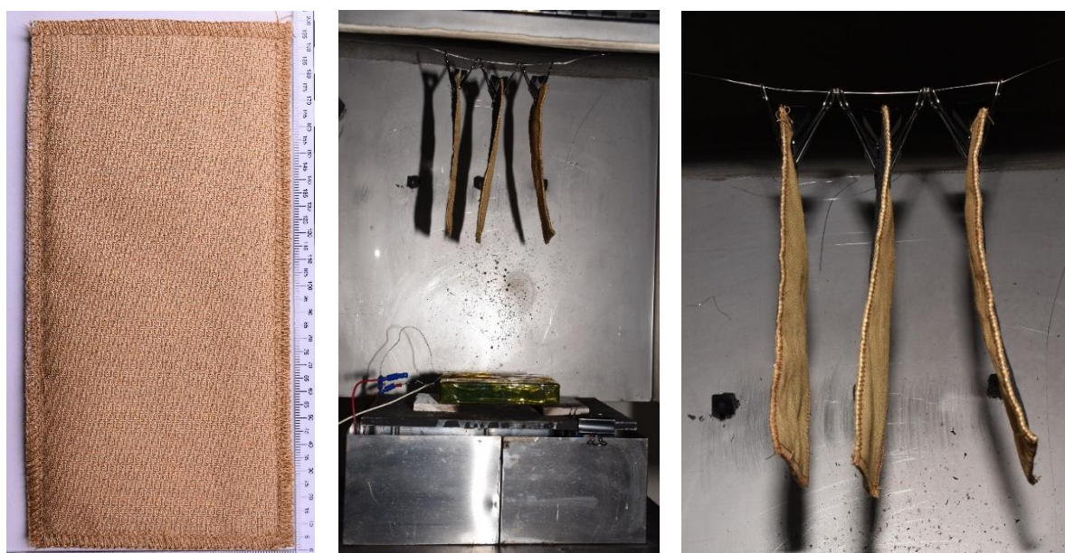
Figure 89. Example images of PPC swatches and arrangement within test chamber.
