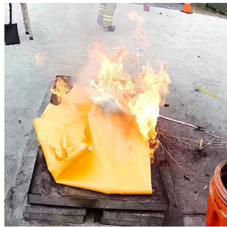
Figure 70. The battery in test 'Test 22: Aluminium, LiB fire blanket' prior to the application of the LiB blanket and 4 s after application, a jet flame burned through.
