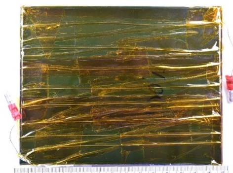
Figure 88. Prepared LFP LiB cell for PPC decontamination tests.
