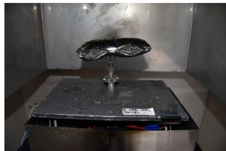
Figure 7. NMC pouch cell at 30% SoC under nail penetration abuse. Cell deformation has occurred, but the outside of the cell casing was still relatively intact.
