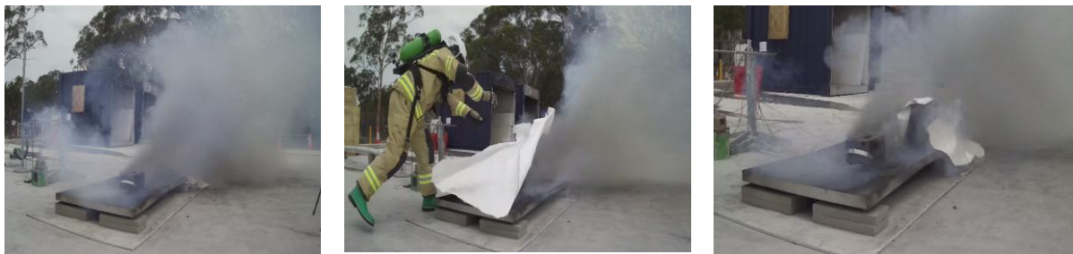
Figure 69. The high volume and pressure of venting making application of the fire blanket difficult (Test 35: Steel, Standard fire blanket').
