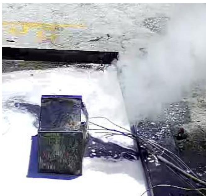
Figure 57. The battery casing opening along the seam. Encapsulating agent can be seen to pool in the case as water vapour continues to be emitted ('Test 44: Steel, Encapsulating agent').
